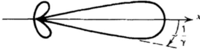
Figure 1.2.: Angular distribution of the radiation of a particle whose acceleration is perpendicular to its velocity. Taken from Rybicki & Lightman (1979)
